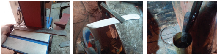
Figure 3: Demonstration of grinding, shape cutting and hardening in oil
