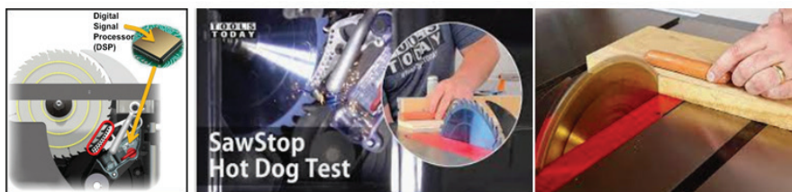
Figure 5. SawStop passive safety system for table saw, [7]
