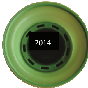
Figure 3. Indication of the year of manufacture of the diaphragm of the pulmonary automaton, manufacturer MSA
