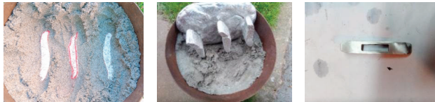
Figure 4: Shield mould making, casting and final shape after sanding
