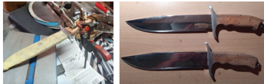
Figure 5: Glued shield to the body and final shape after grinding
