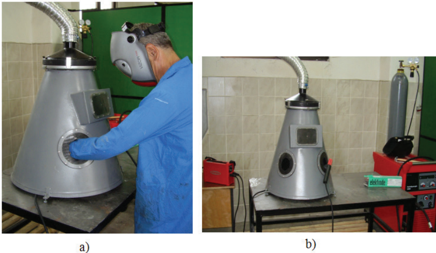
Figure 1. a) The welding chamber and the position of the welder during the experiment, b) The welding chamber and the welding machine
