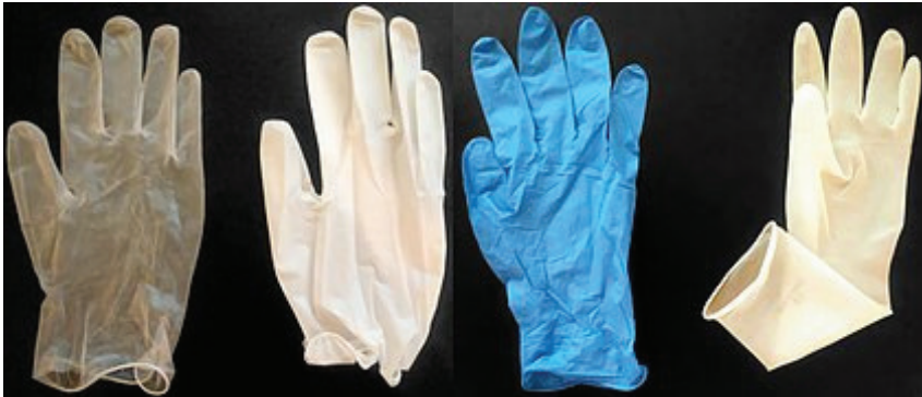
Figure 2. Gloves of various materials, from left to right from the least elastic to the most elastic- Vinyl, Elastic Vinyl, Nitrile and Latex (Picture source: Wikimedia Commons)
