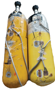
Figure 2. Detection of dilatations on a medical air accumulator
