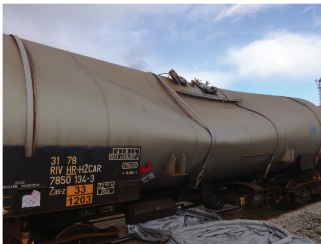
Figure 1: Deformed tank wagon due to the negative pressure (vacuum). [4]
