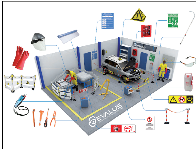
Figure 1: High voltage work area [1]
